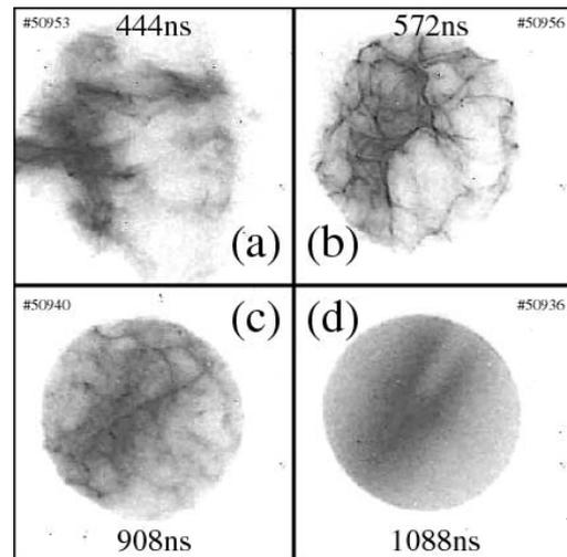
**FIGURE 4.** Typical shadowgraph after an IREB passed through. (a)  $\delta = 444$ ns, (b)  $572$ ns, (c)  $908$ ns, and (d)  $1088$ ns. The plasma density is  $2 \times 10^{11} \text{cm}^{-3}$ , and the beam density is about  $10^{10} \text{cm}^{-3}$ .
