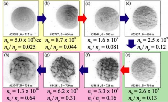
**FIGURE 6.** The beam density is decreased with keeping plasma density constant,  $\tau=100 \mu\text{s}$ .
