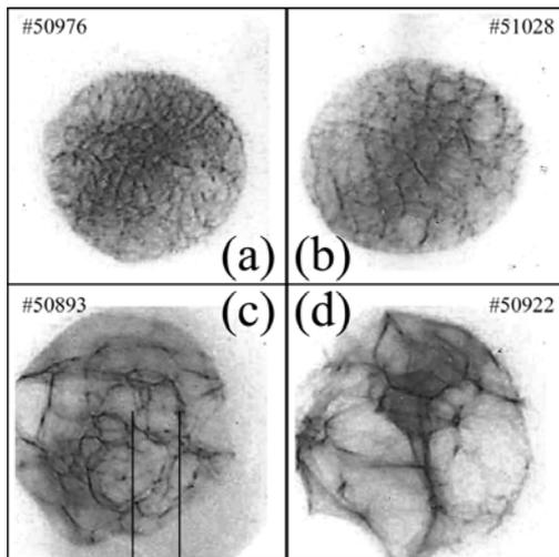
**FIGURE 3.** The plasma density dependence. (a)  $\tau = 50 \mu$ s, (b)  $60 \mu$ s, (c)  $80 \mu$ s, (d)  $100 \mu$ s. The diameter of the hole is measured from one mesh to the next mesh, which is mentioned as the mesh size,  $b$ , in this paper.
