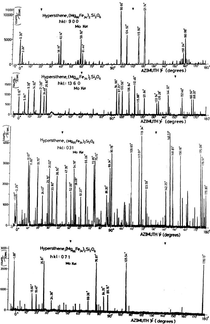
Fig. 2. The 900, 13 6 0, 031 and 071 reflections are step-scanned in  $\psi$ -azimuth from  $-2.0$  to  $180.0$  degrees at intervals of  $0.04$  degrees. The true intensity is corresponded with the background level. Near the position of symmetrical setting, these reflections have also strong spectra. These spectra can be turned down at intervals of  $90$  degrees.
