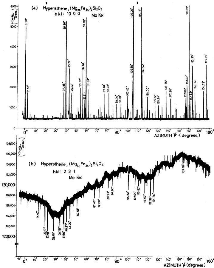
Fig. 3. (a) The Umweganregung peaks appear in intrinsic 10 0 0 intensity. The true intensity is background level with about 500 counts per 20 seconds. (b) Integrated intensities undergoing multiple diffractions (Umweganregung and Aufhellung) and anisotropic extinction (wave-swelling absorption) for the 231 reflection are shown.
