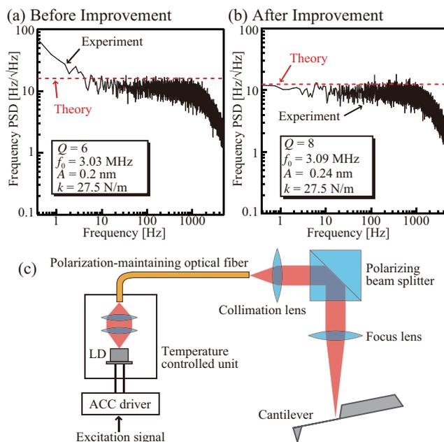
**Fig. 2.** (Color online) (a, b) FM spectra obtained with a USC cantilever in water before and after the improvement of the photothermal excitation setup. (c) Improved setup for the photothermal excitation. Reused with permission from Ref. 18. Copyright 2012 IOP Publishing.
