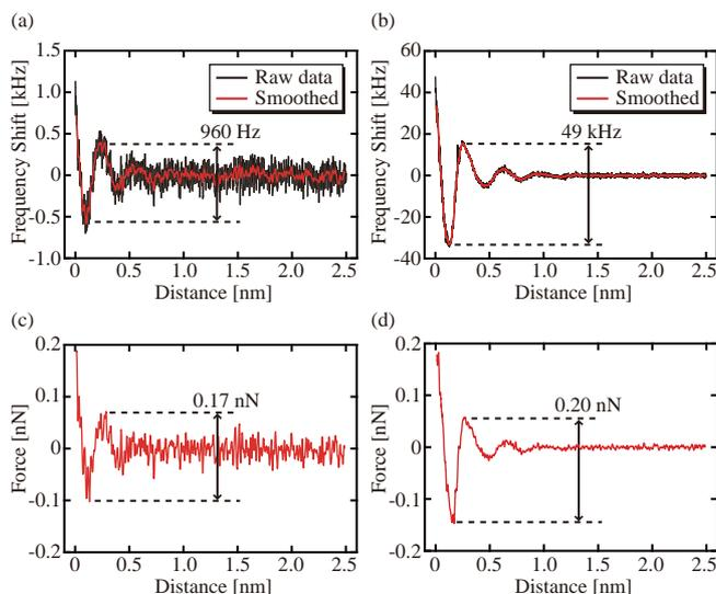
**Fig. 4.** (Color online) (a) (b) Frequency shift versus distance curves measured on a cleaved mica surface in PBS solution with NCH and USC cantilevers, respectively. Sampling rate: 2 kHz. Tip velocity: 1 nm/s.  $B = 100$  Hz. (c) (d) Force versus distance curves calculated from the frequency shift curves shown in (a) and (b), respectively. Reused with permission from Ref. 18. Copyright 2012 IOP Publishing.
