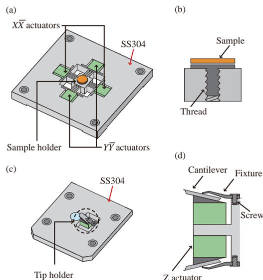
**Fig. 5.** (Color online) Schematic illustrations of the separate-type high-speed scanners. (a)  $XY$  sample scanner. (b) Sample holder using the screw holding mechanism. (c)  $Z$  tip scanner with a counter balance actuator. (d) Cantilever holder with a plate spring and a screw. Reused with permission from Ref. 39. Copyright 2013 AIP Publishing.
