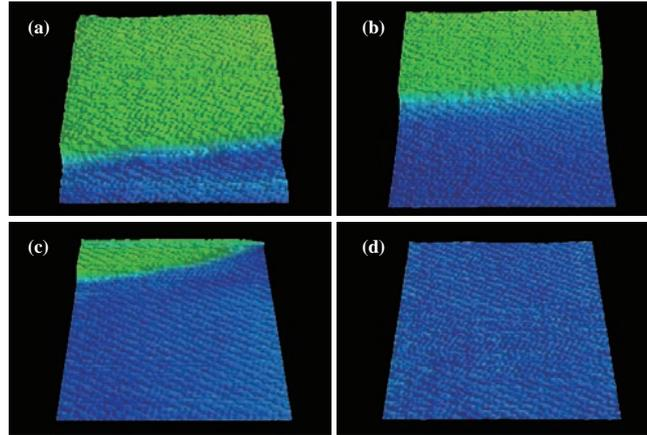
**Fig. 8.** (Color online) Successive PM-AFM images of calcite crystal dissolution process in water: (a) 0, (b) 20, (c) 32, and (d) 40 s. Scan size:  $20 \times 20 \text{ nm}^2$ . Scan rate: 250 Hz. Imaging speed: 2 s/frame. Pixel size:  $500 \times 500 \text{ pix}^2$ . Tip velocity:  $10 \mu\text{m/s}$ . Reused with permission from Ref. 40. Copyright 2014 AIP Publishing.
