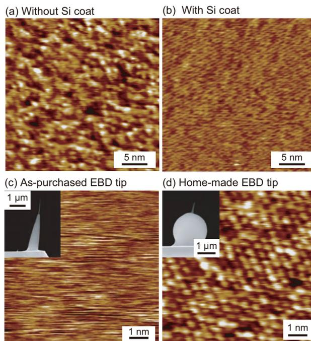
**Fig. 3.** (Color online) FM-AFM images of a cleaved mica surface obtained in PBS solution using a USC cantilever. (a) Without Si coat 30 min after the tip immersion into the imaging solution. (b) With Si coat 200 min after the tip immersion into the imaging solution. (c) As-purchased EBD tip with Si coat. (d) Home-made EBD tip with Si coat. Reused with permission from Ref. 34. Copyright 2015 IOP Publishing.
