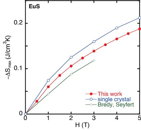
Figure 5: Maximum differential entropy  $-\Delta S_{\max}$  of sintered compacts and single crystal EuS induced by several magnetic fields. Density  $\rho = 5.75 \text{ g/cm}^3$  is used to convert the single crystal data.
