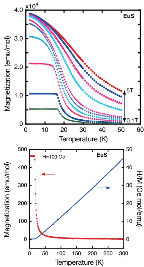
Figure 1: (Upper panel) Magnetization of sintered EuS as functions of temperature in magnetic fields of 0.1, 0.2, 0.4, 0.6, 0.8, 1, 2, 3, 4, and 5 T. (Lower panel) Magnetization and inverse susceptibility of sintered EuS at 100 Oe versus temperature.
