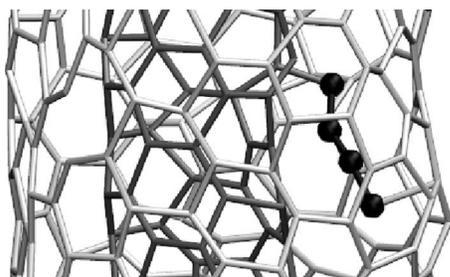
FIG. 7. Snapshot of the typical geometry for interstitials (black atoms) from a simulation with a curvature radius of 40 Å at 4000 K.
