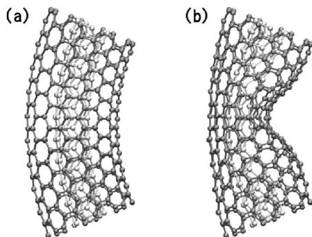
FIG. 1. (a) Initial atomic configuration of DWNT with a curvature radius of 30 Å and (b) final state after 3.0 ps. The inner and outer tube have chiralities of (3,3) and (8,8), respectively.
