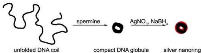
**Figure 1.** Schematic representation of the silver nanorings synthesis: Unfolded DNA chain, DNA toroidal condensate formed after the addition of a condensing agent (in this study, spermine, noted  $\text{SPM}^{4+}$ , a tetravalent polycation) and DNA-templated silver nanorings (silver shell is shown as red) formed after  $\text{Ag}^+$  reduction by  $\text{NaBH}_4$ .
