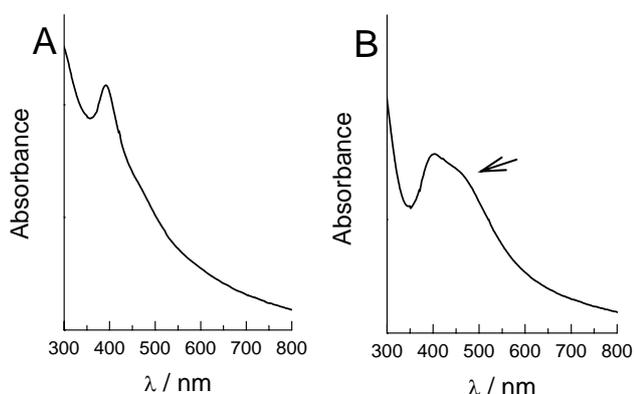
**Figure 4.** UV-Vis spectra of the control solution without DNA (A) and the silver nanorings solution (B). The arrow indicates the characteristic long wavelength absorption shoulder (470 nm) inherent to the silver ring morphology.
