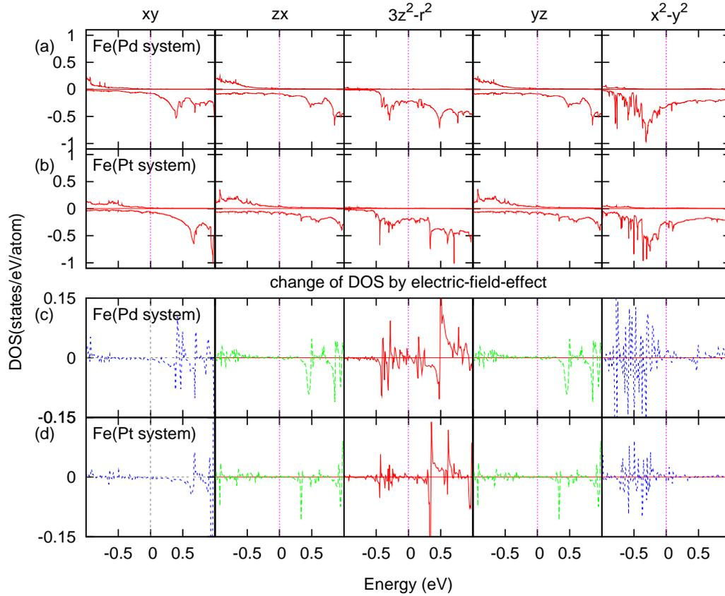
**Figure 5.** (color online). The local density of states for Fe 3d components in (a) Pd/Fe/Pd(001) and (b) Pt/Fe/Pt(001) at zero electric field and the electric-field induced change in (c) Pd/Fe/Pd(001) at 9.6V/nm and (d) Pt/Fe/Pt(001) at 4.7V/nm. The vertical lines indicate the Fermi level.
