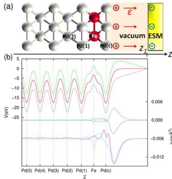
**Figure 1.** (color online)(a) Schematic view of the calculation model for the surface, Pd/Fe/Pd(001). (b) The upper curves present the planar-averaged electrostatic potential along  $z$ -coordinate at  $\mathcal{E} = -9.6$  (green dashed curve),  $0.0$  (red solid curve), and  $9.6$  (blue dotted curve) V/nm. The lower curves present the EF-induced electron densities for majority-spin (magenta dotted curve) and minority-spin (cyan dotted curve) states at  $9.6$  V/nm.
