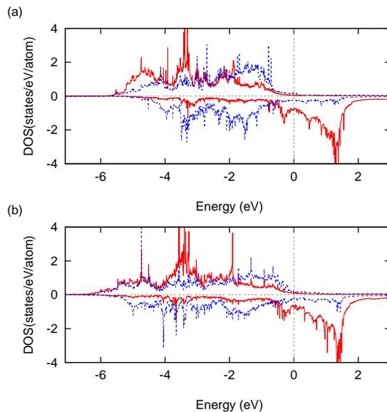
**Figure 4.** (color online). The local density of states for (a) Pd/Fe/Pd(001) and (b) Pt/Fe/Pt(001). The red full and blue dashed curves indicate the  $d$ -component of Fe and that of the capping metal (Pd or Pt), respectively.
