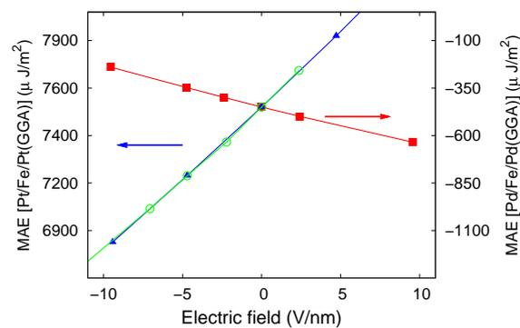
**Figure 2.** (color online). Magnetic anisotropy energies (MAEs) for electric fields: Pd/Fe/Pd(001)(GGA)(red squares) and Pt/Fe/Pt(001)(GGA)(blue triangles), in comparison with Pt/Fe/Pt(001)(LDA)(green circles) [13].
