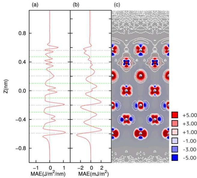
**Figure 3.** (color online). Electric field induced change of the magnetic anisotropy energy (MAE) densities at 9.6V/nm; (a) the planar-averaged MAE density  $\Delta(z)$ , (b) the function  $T(z)$  obtained by integrating (a) along  $z$ -direction, (c) the MAE density map on the (110) plane which contains the Fe and Pt atoms. The horizontal thin and thick dashed lines in (a) and (b) indicate the atomic  $z$ -coordinates and the layer boundaries (intermediate of  $z$ -coordinates), respectively.
