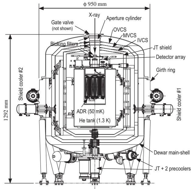
Figure 3: Cross section of the SXS dewar.
