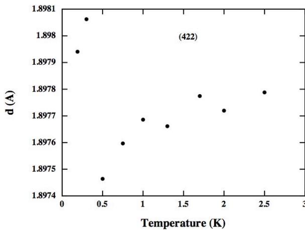
**Figure 5,** Temperature variation of lattice space  $d$  for (422) x-ray reflection of  $\text{PrOs}_4\text{Sb}_{12}$ .
