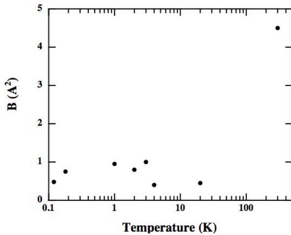
**Figure 3.** Temperature variation of  $B$  parameter of  $\text{PrOs}_4\text{Sb}_{12}$ .
