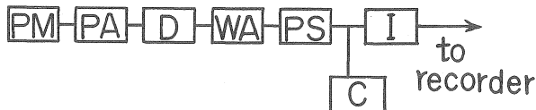
Fig. 2. Block diagram of photon counting system. PM: Photomultiplier, PA: Preamplifier, D: Discriminator, WA: Wide band amplifier, PS: Pulse shaper, C: Counter, I: Integrator.
