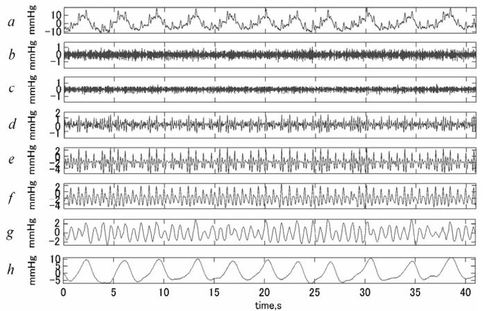
Fig. 3 Wavelet decompositions of pressure signal from the sensor in near-neck occiput region. (a) Raw signal (near-neck occiput pressure). (b)-(g) Waveforms from detail components in  $2^j$  ( $j=1-6$ ) scales, respectively. (h) Waveforms from approximation components in  $2^6$  scale.
