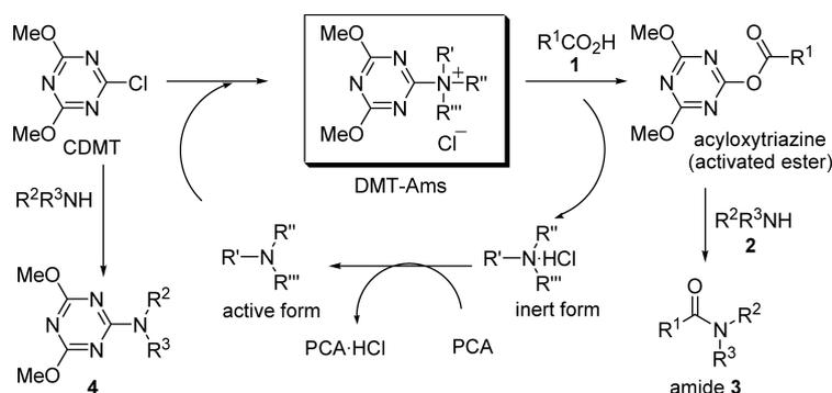
Chart 1. Catalytic Amide-Forming Reaction Involving DMT-Am
