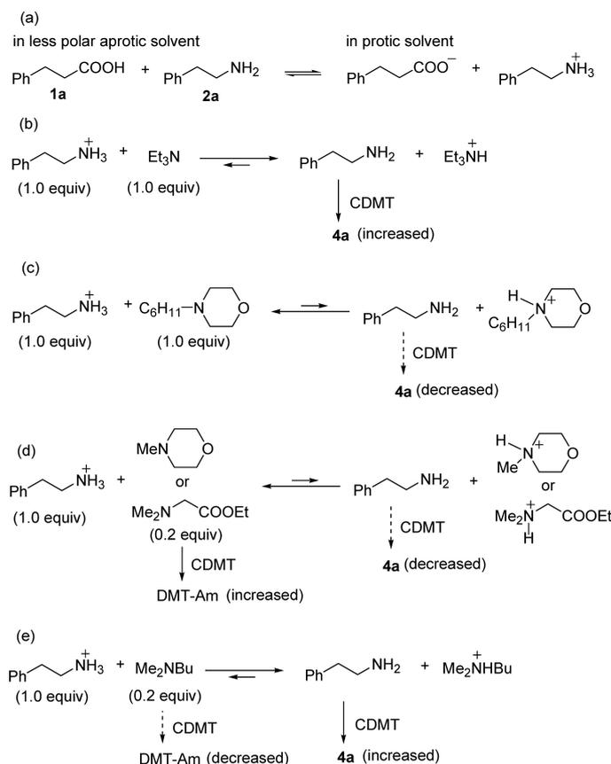
Chart 3. Mechanistic Consideration for the Effect of Acid–Base Equilibrium of Reactants on the Products Distribution in Aqueous Solvents
