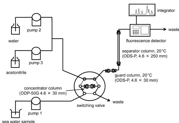
Fig. 1. Schematic Diagram of the Proposed System
