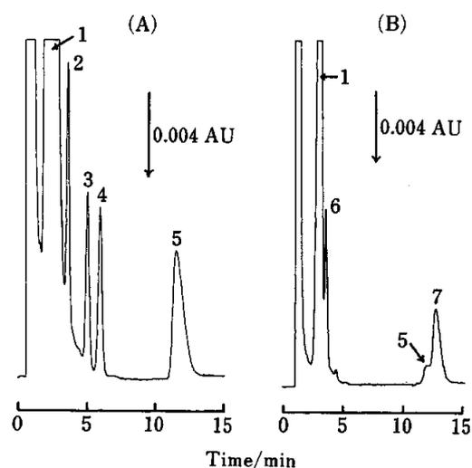
Fig. 2 Chromatograms of (A) inorganic anions and (B) carboxylates. Sample: (A) a 100 ml mixture of chloride, bromide, nitrate and sulfate (each  $1.0 \times 10^{-7}$  M); (B) 20 ml of butyrate and tartrate ( $5.0 \times 10^{-7}$  M). Peaks: 1, hydrogencarbonate; 2, chloride; 3, bromide; 4, nitrate; 5, sulfate; 6, butyrate; 7, tartrate.
