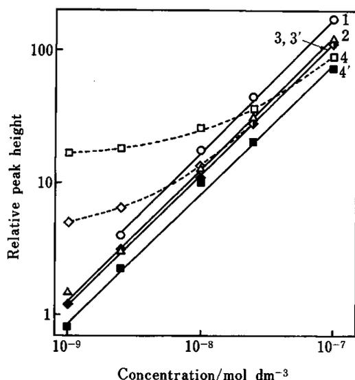
Fig. 3 Calibration curves. Sample: a mixture of chloride, bromide, nitrate and sulfate. Loading volume: 100 ml. Lines: 1, chloride; 2, bromide; 3, nitrate; 4, sulfate; 3' and 4', background-corrected lines of 3 and 4, respectively.
