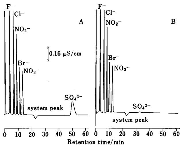
Fig. 1 Comparison of counter ion effect between Bis-Tris (A) and Trien (B) on retention times of analyte anions (see text for the analytical conditions). Sample: 20  $\mu$ l of a solution containing 10 ppm of each of the indicated anions.
