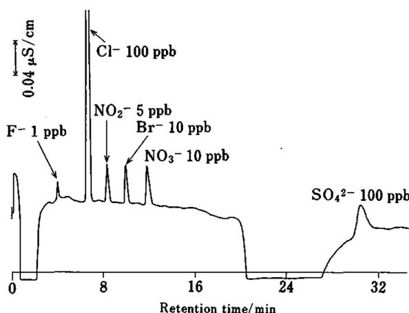
Fig. 2 Chromatogram of trace amount of anions (analytical conditions were the same as these of B in Fig. 1). Sample: 1 ml of a solution containing the indicated anions.
