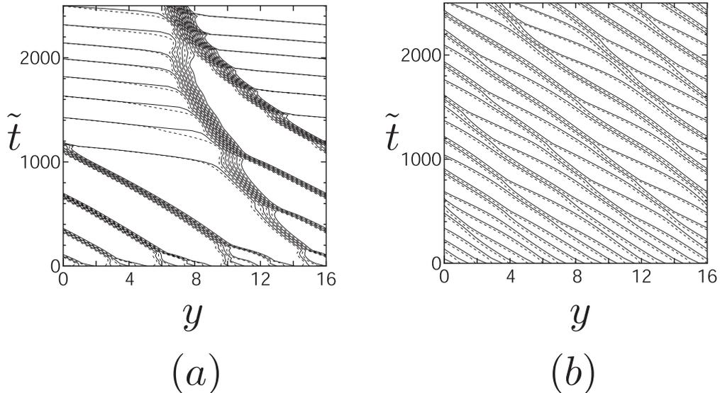
FIG. 9: Time evolution of step positions with a large evaporation rate with (a) step-down drift and (b) step-up drift. Parameters are  $|f| = 0.1$ ,  $D_B = 1$ ,  $D_A = 0.1$ ,  $\tilde{A}_2 = 10^{-4}$  with  $\nu = 2$  and the lifetime  $\tau = 50$ . The number of steps is 32.
