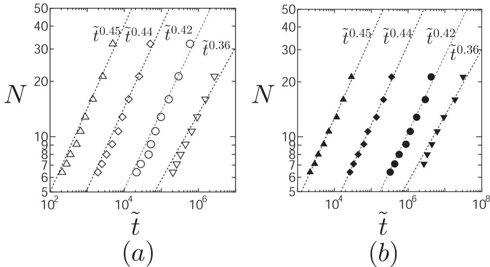
FIG. 6: Time dependence of the bunch size with various repulsive potential with (a) step-down drift and (b) step-up drift. The exponent of the repulsive potential is  $\nabla \nu = 0$ ,  $\circ \nu = 2$ ,  $\triangle \nu = 4$  and  $\diamond \nu = 6$ .
