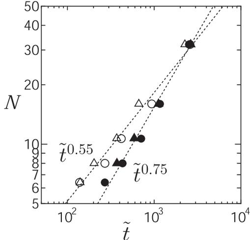
FIG. 8: Time dependence of bunch size in sublimation with the potential of  $\nu = 0$  and of  $\nu = 2$ . The parameters are the same as in Fig. 7 for  $\nu = 2$ . For  $\nu = 0$ ,  $\tilde{A}_0 = 10^{-2}$  and other parameters are the same as in Fig. 7. The open marks indicate step-down drift ( $\Delta$   $\nu = 0$  and  $\circ$   $\nu = 2$ ), and filled marks indicate step-up drift.
