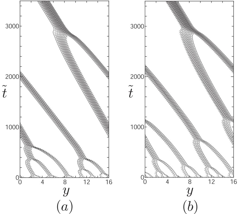
FIG. 7: Time evolution of step positions in sublimation with (a) step-down drift and (b) step-up drift. Parameters are  $f = 0.2$ ,  $D_B = 2$ ,  $D_A = 1$ ,  $\tilde{A}_2 = 10^{-4}$  with  $\nu = 2$  and the lifetime  $\tau = 80$ . The number of steps is 32 and the initial step distance is 0.5.
