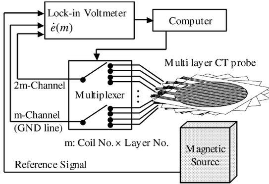
Fig. 4. Measurement system of full electronic magnetic CT probe.
