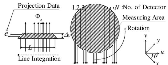
Fig. 2. Two-dimensional magnetic CT probe [3] and its principle.
