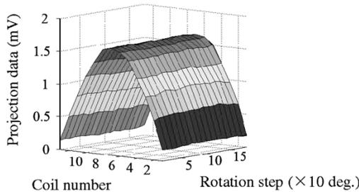
Fig. 7. Projection data of spherical magnetic CT probe.
