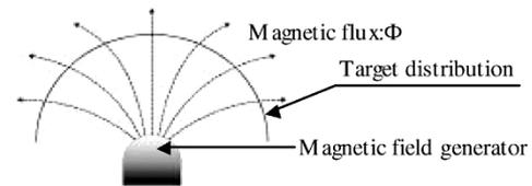
Fig. 1. Measuring target of magnetic flux distribution.
