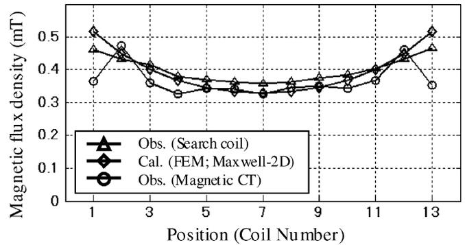
Fig. 9. Comparison between measured data and FEM result.
