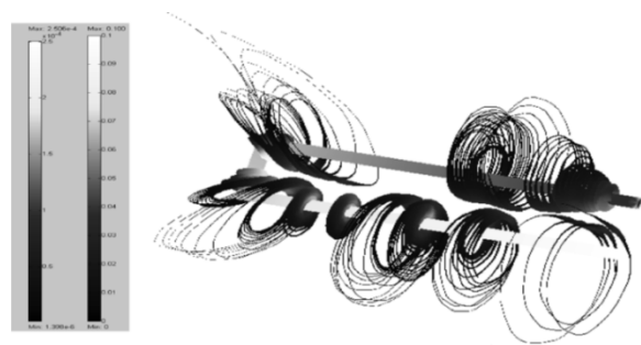
Fig. 4. Magnetic flux lines for meander sensor obtained from the FE model.
