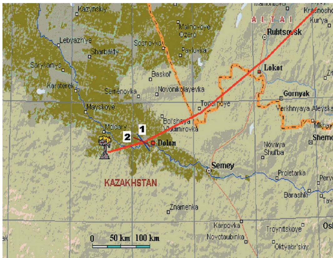
**Fig. 1.** Regional map showing the SNTS and populated areas. The solid thick line represents the roughly estimated central axis of the radioactive trace of the 29 August, 1949 nuclear test<sup>1)</sup>; 1 represents the cross section of aerial exposure rate measurements near Dolon village<sup>1)</sup>; 2 represents the cross section of ground exposure rate measurements near Dolon village<sup>1)</sup>.
