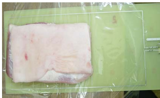
Figure 1. The interdigital sensor and pork belly cuts
