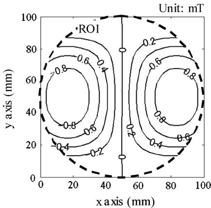
Fig. 3. Model field of 2-D magnetic flux distribution.
