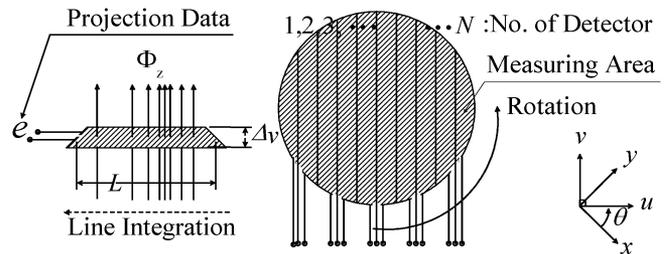
Fig. 1. 2-D magnetic CT probe and its principle.
