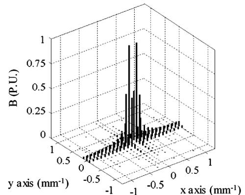
Fig. 5. 2-D Fourier power spectrum. 1 (P.U.) is equal to 0.725 (mT).
