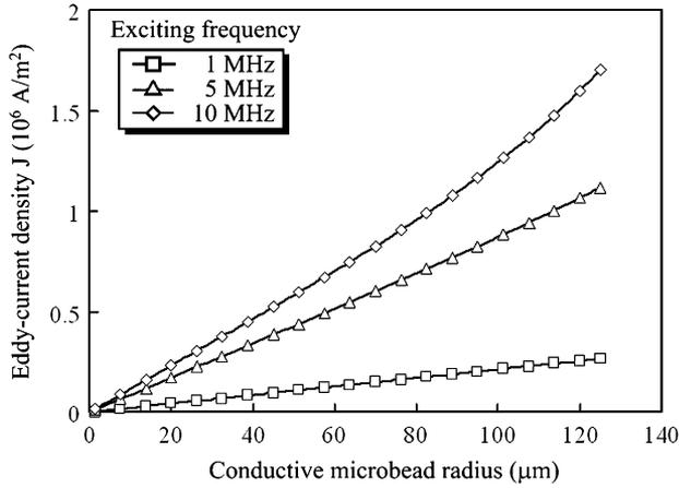
Fig. 3. Eddy-current density distribution in the conductive microbead (PbSn) with 125  $\mu\text{m}$  radius and 162  $\mu\text{m}$  lift-off height.
