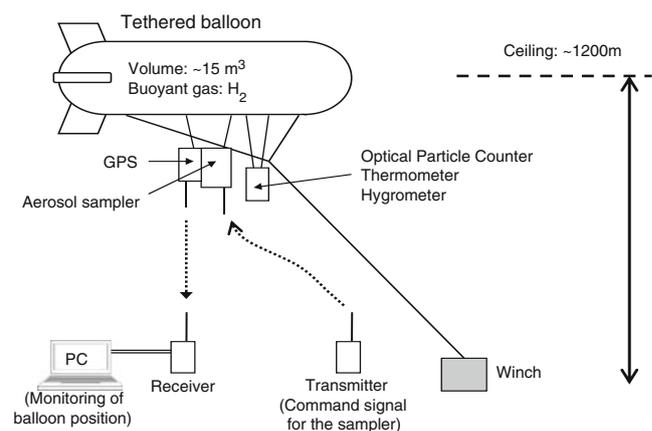
**Fig. 2** Composition of balloon train. Tethered balloon was used to collect dust and micro-bioaerosol particles from the ground to heights of about 1,200 m ( from 1,100 to 2,300 m above sea level). Particle number concentration and size, atmospheric temperature, and humidity were simultaneously monitored
