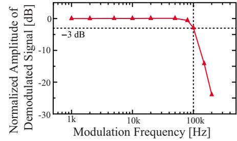
FIG. 2. (Color online) Frequency response of the developed S-PLL. Input signal: 5 MHz  $\pm$  2 kHz, 300 mV<sub>p-p</sub>. The amplitude was normalized with respect to the value at  $f_m=1$  kHz.
