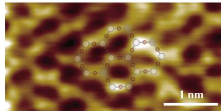
FIG. 4. (Color online) FM-AFM image of a cleaved mica surface in PBS solution (Scan size:  $4 \times 2$  nm<sup>2</sup>, Scan speed: 61 nm/s,  $\Delta f=-390$  Hz,  $A_z=0.22$  nm,  $f_{LPF}=100$  kHz). A Si cantilever (arrow-UHF: Nanoworld) was used ( $f_{CL}=634$  kHz,  $Q=5.8$ ,  $k=27.7$  N/m in liquid). An atomic-scale model of a mica surface is partially overlaid on the image.
