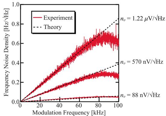
FIG. 3. (Color online) Frequency noise density distribution of the output signal from the developed S-PLL. The input signal is a sum of a clean sine signal and a white noise ( $f_0=500$  kHz,  $A_v=200$  mV,  $f_{LPF}=100$  kHz).
