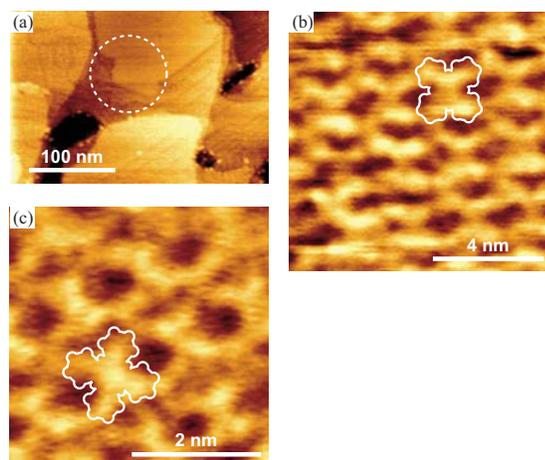
FIG. 4. (Color online) Topographic images of a CoPc monolayer on an Au(111) surface obtained by FM-AFM. (a)  $300 \times 210 \text{ nm}^2$ ,  $\Delta f = -20 \text{ Hz}$ . (b)  $7 \times 7 \text{ nm}^2$ ,  $\Delta f = -260 \text{ Hz}$ . (c)  $4 \times 4 \text{ nm}^2$ ,  $\Delta f = -320 \text{ Hz}$ .
