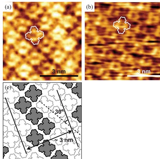
FIG. 2. (Color online) Topographic images of CuPc monolayers on Au(111) surfaces obtained by FM-AFM. (a)  $6 \times 6 \text{ nm}^2$ ,  $\Delta f = -450 \text{ Hz}$ . (b)  $7 \times 7 \text{ nm}^2$ ,  $\Delta f = -134 \text{ Hz}$ . (c) An illustration of molecular arrangements in (a).
