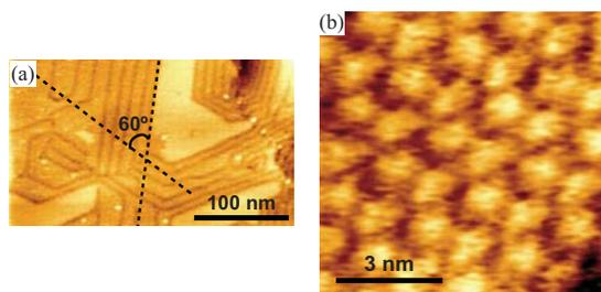
FIG. 3. (Color online) Topographic images of a CoPc monolayer on a Au(111) surface obtained by FM-AFM. (a)  $300 \times 180 \text{ nm}^2$ ,  $\Delta f = -15 \text{ Hz}$ . (b)  $8 \times 8 \text{ nm}^2$ ,  $\Delta f = -380 \text{ Hz}$ .
