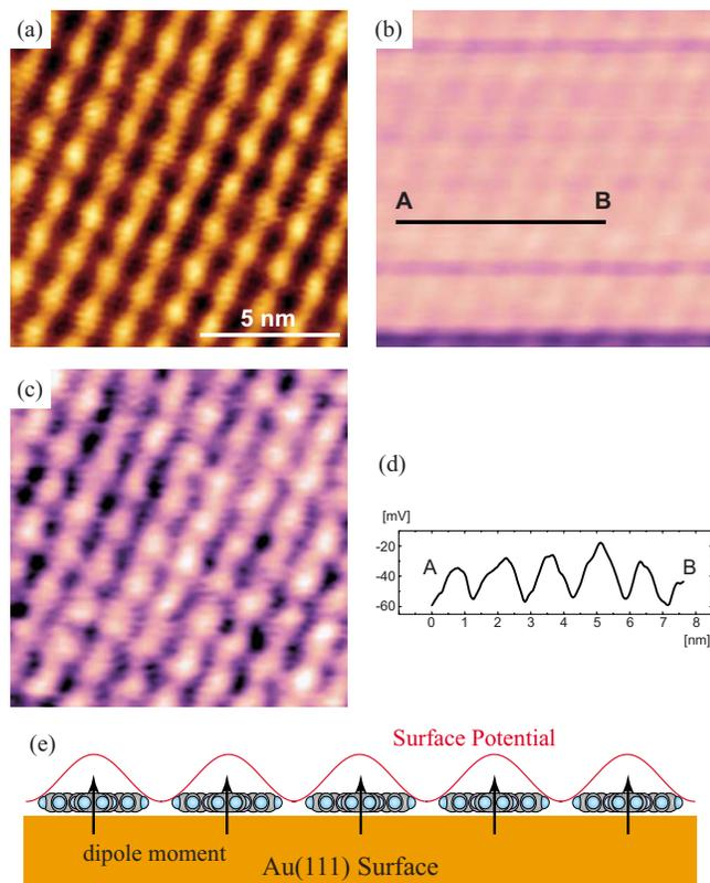
FIG. 6. (Color online) FM-AFM images of a CuPc monolayer on an Au(111) surface,  $12 \times 12 \text{ nm}^2$ ,  $\Delta f = -170 \text{ Hz}$ . (a) Topographic image. (b) SP image. (c) Fluctuation-corrected SP image. (d) A cross-sectional profile measured along the A-B line indicated in (b). (e) A model to explain the molecular-scale SP contrast.
