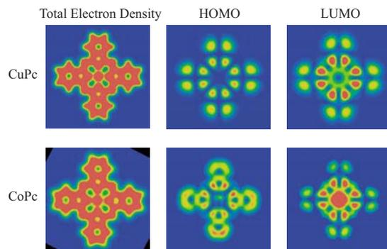
FIG. 5. (Color online) Two-dimensional maps of the total electron density distributions, the electron density distributions of the HOMO, and those of the LUMO at the surface located  $0.25 \text{ nm}$  above the molecular planes of CuPc and CoPc molecules, calculated based on the density functional theory.
