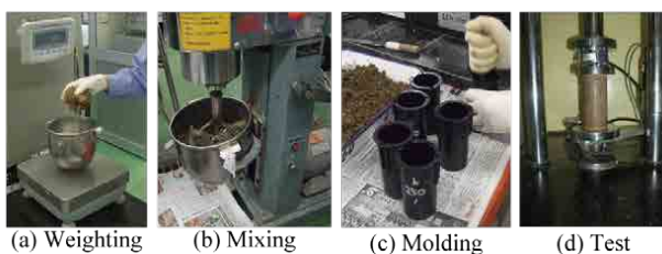
Fig.1 Overview of soil test
