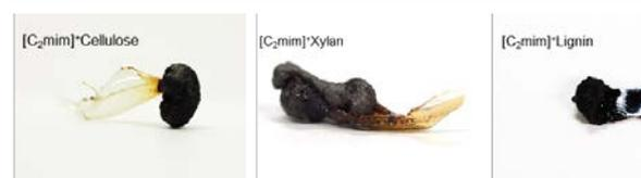
**Fig. 3** Char formation of the thin films of [C<sub>2</sub>mim]<sup>+</sup>cellulose (left), [C<sub>2</sub>mim]<sup>+</sup>xylan (centre), and [C<sub>2</sub>mim]<sup>+</sup>lignin (right) after burning and extinguishing the fire.
