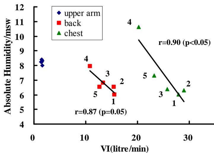
Fig. 5 Relationship between the ratio of average moisture concentration [ $\text{g m}^{-3}$ ] to average sweat rate [ $\text{g min}^{-2} \text{m}^{-2}$ ] and Ventilation Index (VI) over 10 min after the onset of sweating. The numbers represent the samples.
