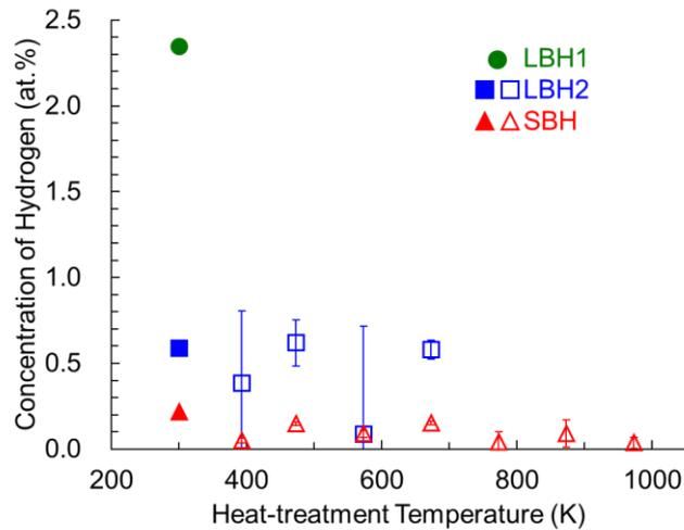
**Fig. 1** Heat-treatment temperature dependence of the concentration of impurity hydrogen atoms in hydrothermally grown ZnO single crystals. The solid symbols represent the data for the as-grown sample.
