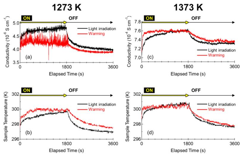
**Fig. 3** Time variations of the conductivities ((a) and (c)) and sample temperatures ((b) and (d)) for the samples heat-treated at 1273 K (left) and 1373 K (right) as a functions of elapsed time of light irradiation (black lines) and of sample warming (red lines).
