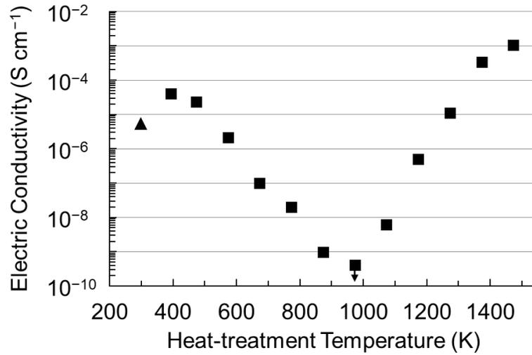
**Fig. 2** Heat-treatment temperature dependence of the electric conductivity in hydrothermally grown ZnO single crystals. The triangle symbol represents the data for the as-grown ZnO sample. The upper limit is shown for the electric conductivity in the sample heat-treated at 973 K.
