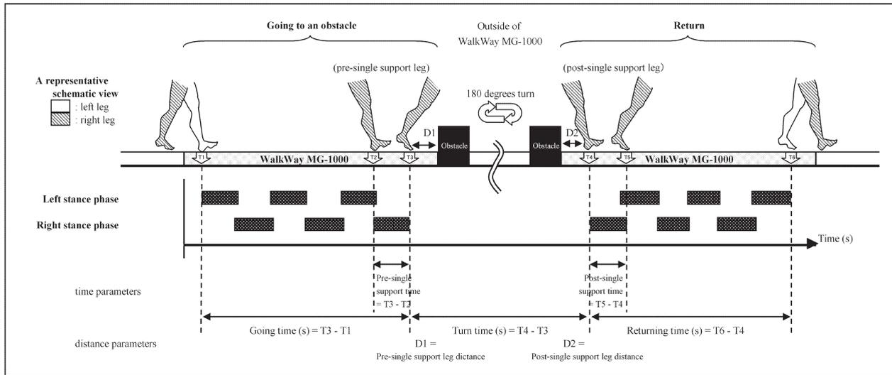
Fig. 2. Explanation of gait parameters of the TUGO test.
