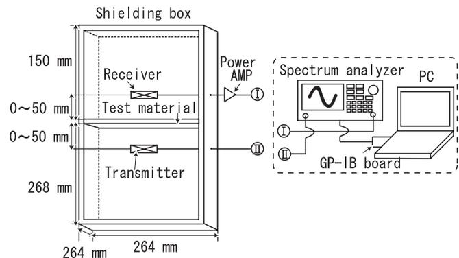
Fig. 1. Estimation system of relative permeability and conductivity
