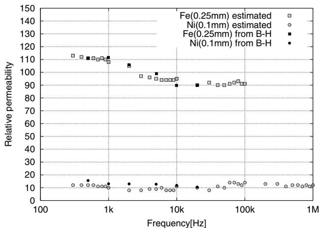
Fig. 5. The frequency characteristics of the relative permeability
