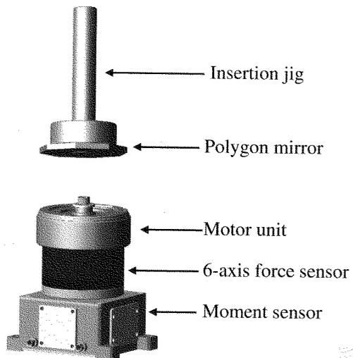
Fig 2: Experimental apparatus
