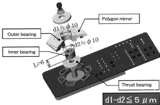
Fig 1: Schematic of the polygon motor unit
