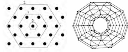
Fig. 4. SOM: hexagonal grid and toroidal map topology.
