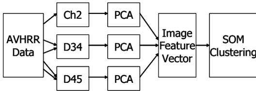
Fig. 2. The diagram of satellite image clustering.
