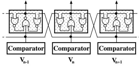
**Fig. 2.** Structure of local maximum detector
