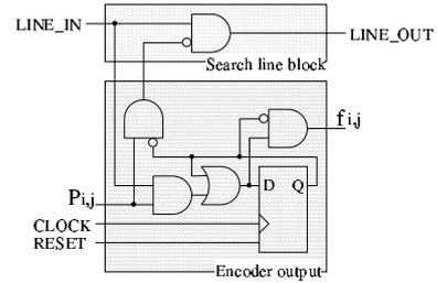
**Fig. 8.** Circuit of the scan path for one pixel
