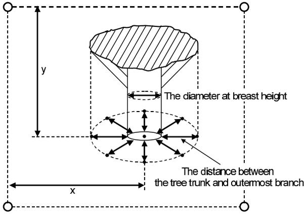
Fig. 2. In the field survey, we measured the tree stand location  $(x,y)$  in the labeled block, distances between the tree trunk and outermost branch in eight directions, and diameter at breast height.
