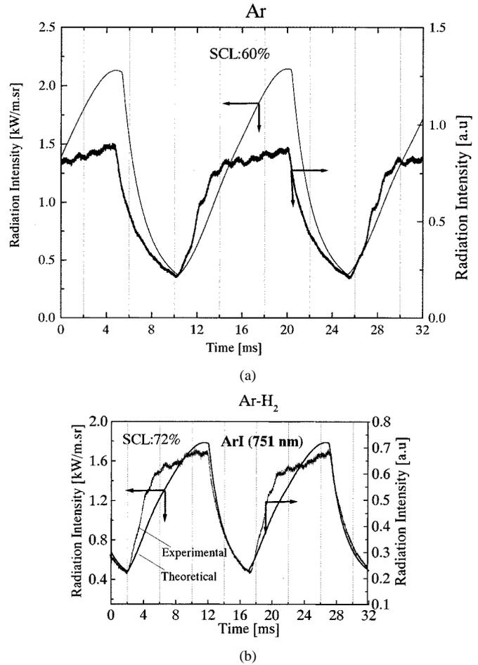
Fig. 12. Comparison of experimental and simulated radiation intensities of ArI (751 nm), for (a) Ar and (b) Ar-H<sub>2</sub> plasmas, measured/predicted at 10 mm below the coil-end ( $z = 2.14$  mm).
