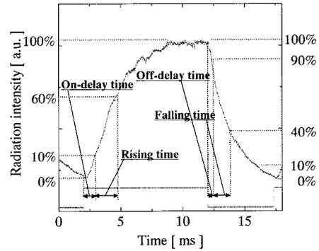
Fig. 8. Definitions of different response times of plasma.
