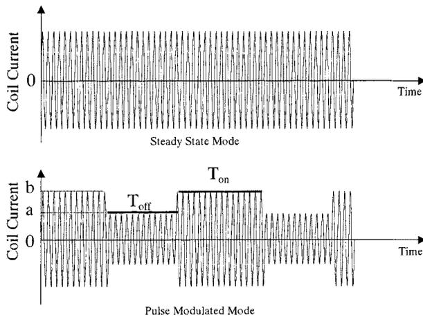
Fig. 1. Concept of pulse-modulated induction thermal plasma.
