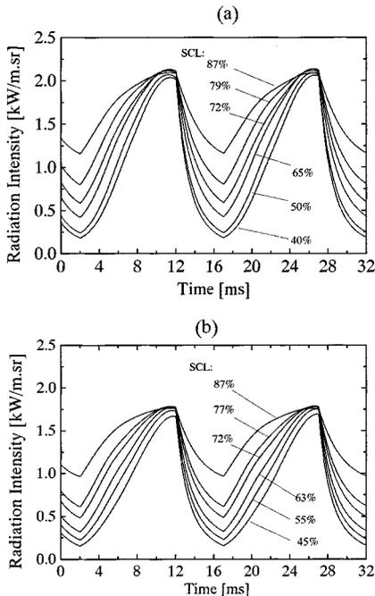
Fig. 7. SCL effect upon time-dependent integrated radiation intensities of ArI (751 nm) for (a) Ar and (b) Ar-H<sub>2</sub> plasmas, predicted at 10 mm below the end coil.
