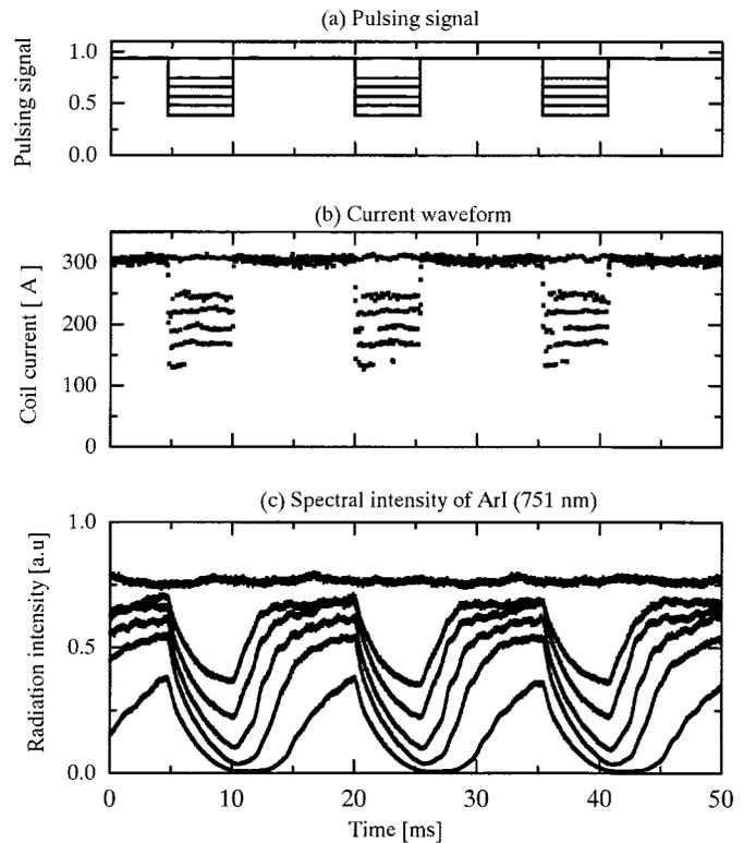
Fig. 10. (a) Spectroscopically measured temporal pulsing signal, (b) modulated current waveform peaks, and (c) radiation intensity of atomic argon at 10 mm below the end coil for Ar-H<sub>2</sub> plasma.
