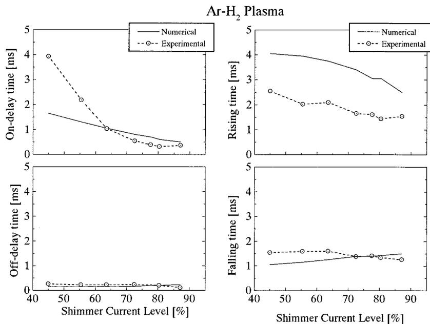
Fig. 14. Comparison of experimental and simulated response times of Ar-H<sub>2</sub> plasma measured/predicted at 10 mm below the coil-end ( $z = 214$  mm).
