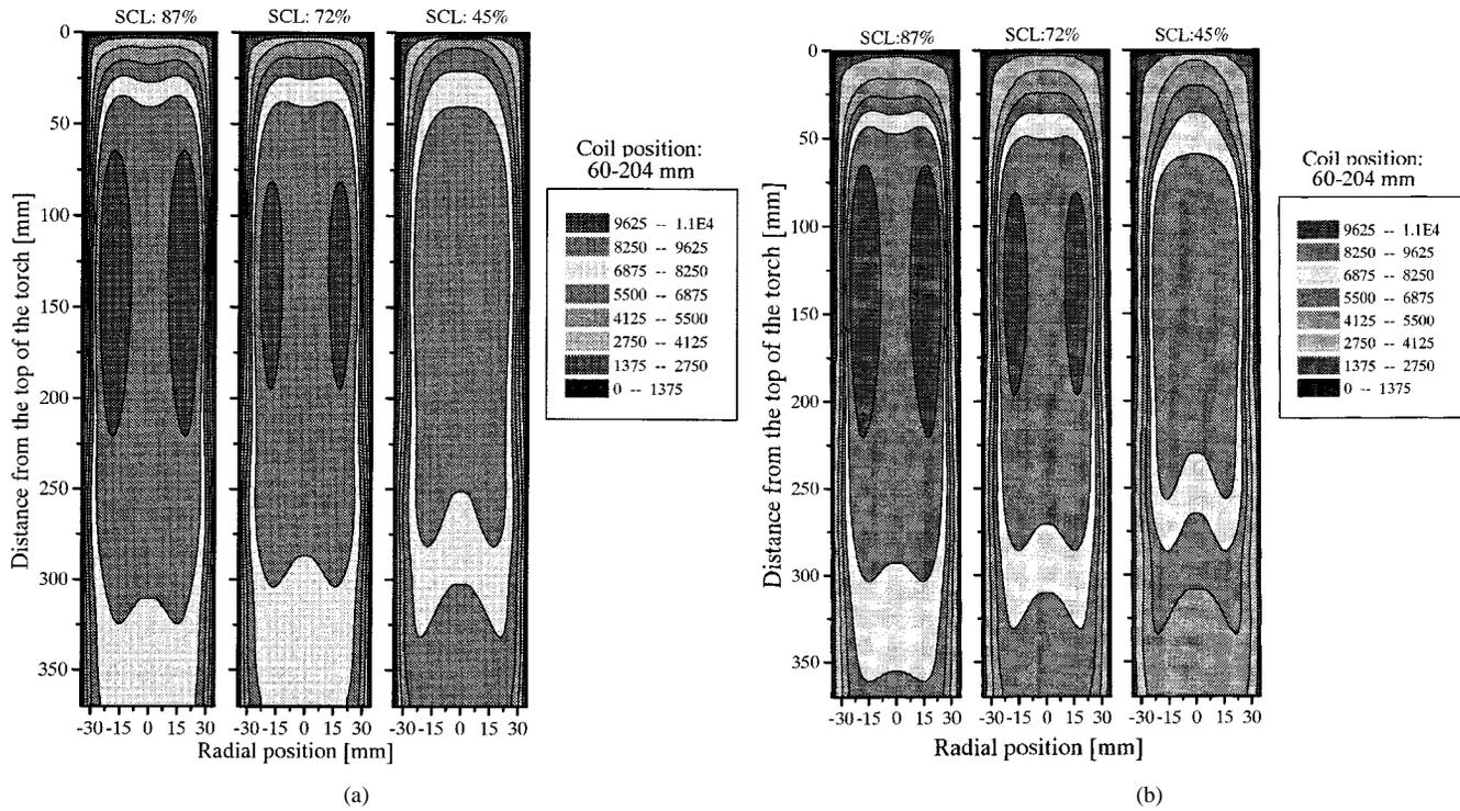
Fig. 4. SCL effect upon the spatial temperature distributions of Ar (a) and Ar-H<sub>2</sub> (b) plasmas predicted at the end of off-pulse.
