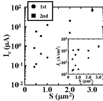
Fig. 5. Junction area  $S$  dependence of critical currents  $I_c$  estimated from 1st (circle) and 2nd (square)  $I_c$  of IJJs at 4.2 K. The inset shows  $S$  dependence of critical current density  $J_c$  for same junctions.
