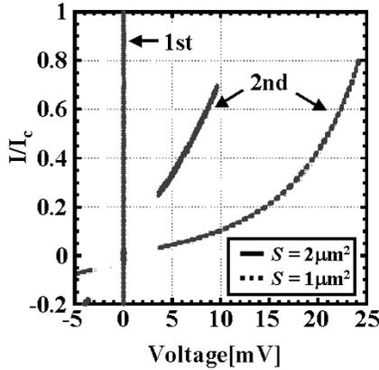
Fig. 2. Normalized current-voltage characteristics on low bias region for IJJs with junction area  $S = 1 \mu\text{m}^2$  and  $2 \mu\text{m}^2$ . The temperature is 4.2 K.
