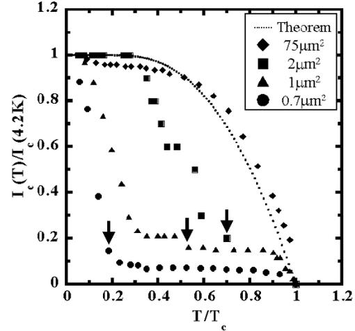
Fig. 3. Temperature dependence of normalized critical currents of IJJs with various  $S$ . Theoretical curve estimated from A-B relation is also plotted. The arrows indicate the threshold temperature  $T_t$ , which corresponds to  $E_J/k_B$  for each IJJs.
