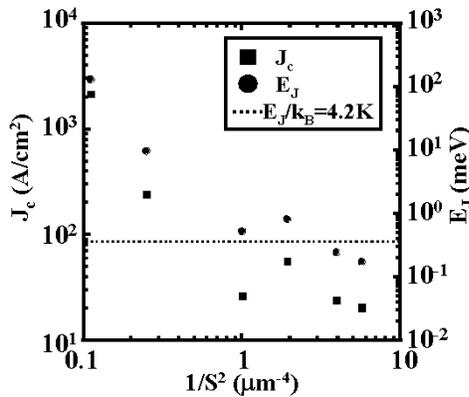
Fig. 6.  $1/S^2$  ratio dependence of critical current density  $J_c$  and Josephson coupling energy  $E_J$ .  $J_c$  and  $E_J$  were estimated from 1st  $I_c$  of IJJs at 4.2 K. The dashed line indicates  $E_J/k_B = 4.2$  K.
