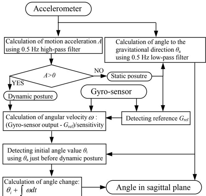
Fig. 2. Algorithm for calculating angle in sagittal plane.
