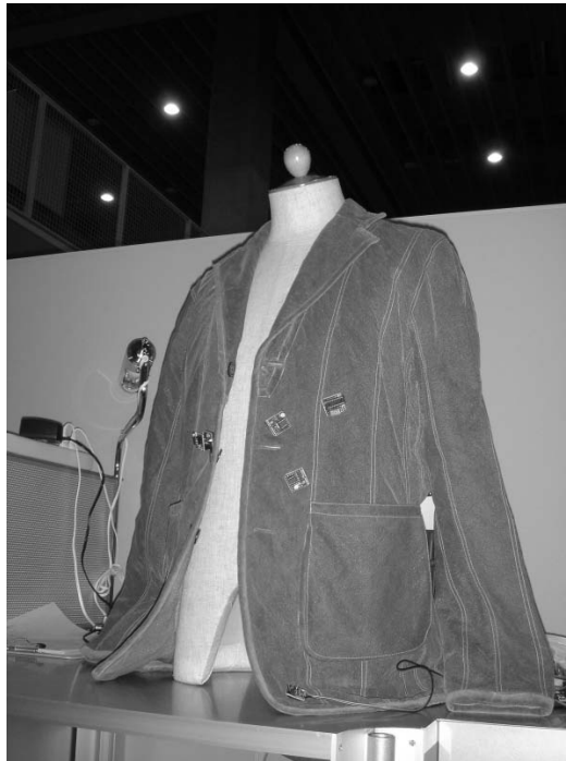
Fig. 2. Developed wear using conductive fabric.
