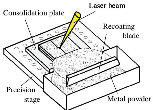
Fig. 1 Schematic illustration for consolidating metal powder
