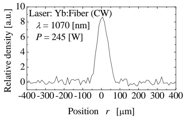
Fig. 2 Profile of laser beam
