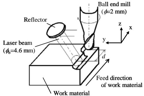
Fig.3 Experimental set up for laser assisted milling
