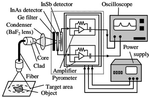
Fig.4 Schematic illustration of two-color pyrometer
