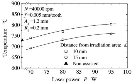
Fig.7 Influence of laser power  $P$  on tool temperature
