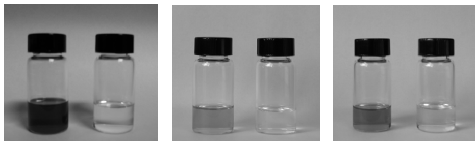
Figure 3. Demonstration of the encapsulation property of 3b in \text{CHCl}_3 toward rose bengal (left), alizarin yellow (center), and thymol blue (right). The left vials in each picture include 3b , while the right vials are the control experiment in the absence of 3b .
