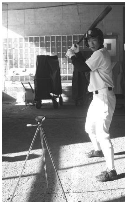
Figure 1 Measurement of bat swing speed using a microwave -type speed measuring instrument
