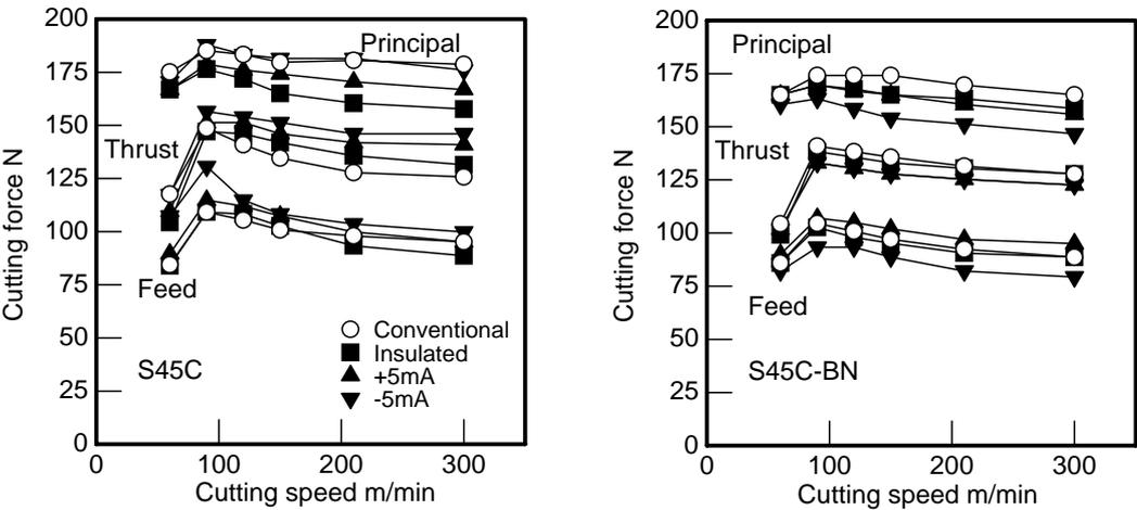
Fig. 4 Relationship between the cutting speed and the cutting force when turning tested steels under various electric conditions
