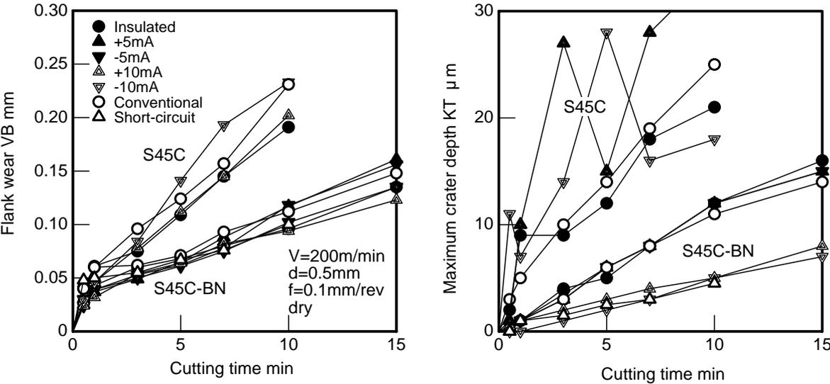
**Fig. 3** Wear progress curves of carbide tool P30 when turning S45C and S45C-BN under following conditions, conventional, insulated, short-circuit and with additional current at the cutting speed 200 m/min
