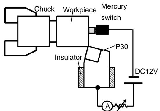
**Fig. 2** Schematic of experimental set up (positive direction)
