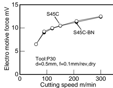
**Fig. 1** EMF in turning of two tested workmaterials with carbide tool P30 for various cutting speed
