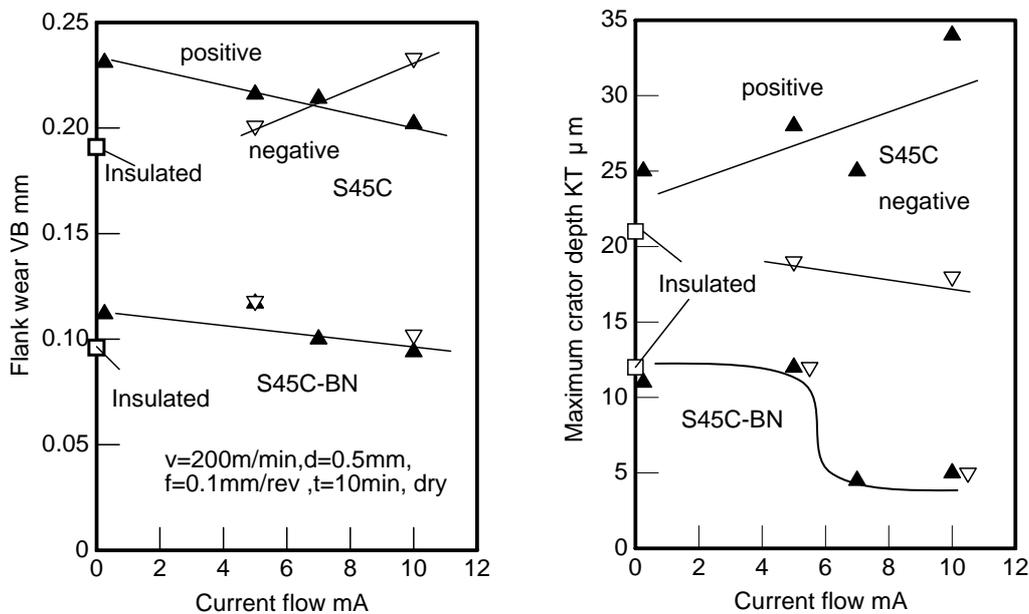
**Fig. 6** Relationship between the tool wear of carbide tool P30 and the current flow in closed circuit when turning S45C and S45C-BN at the cutting speed 200m/min for 10 min
