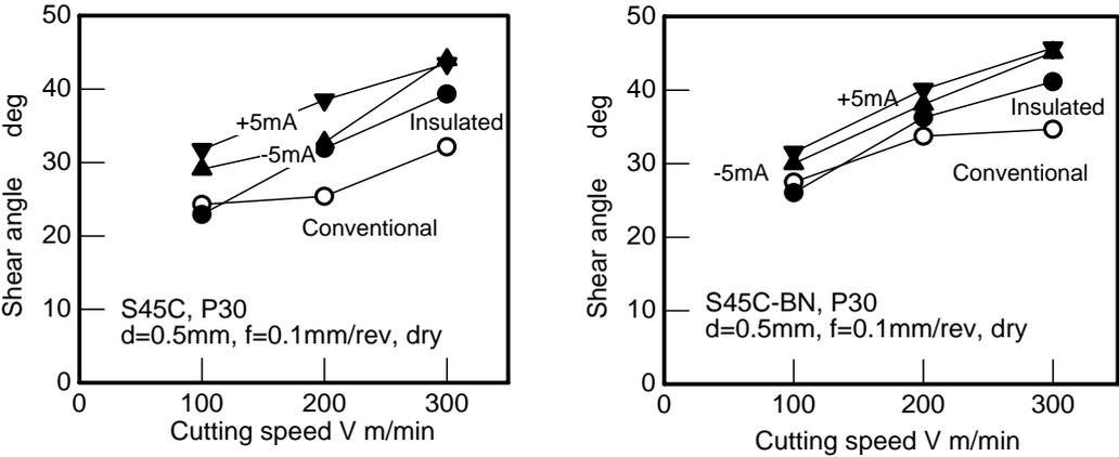
Fig. 5 Shear angle when turning S45C and S45C-BN with P30 carbide tools under various electric conditions
