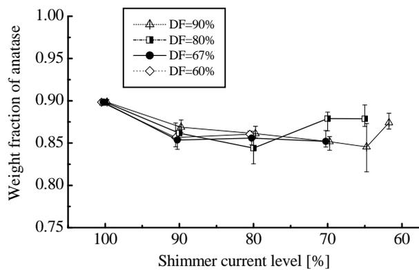
Figure 6: Dependence of the weight fraction of anatase-TiO<sub>2</sub> nanoparticles on the shimmer current level (SCL) at different duty factors (DF) in modulated coil current.
