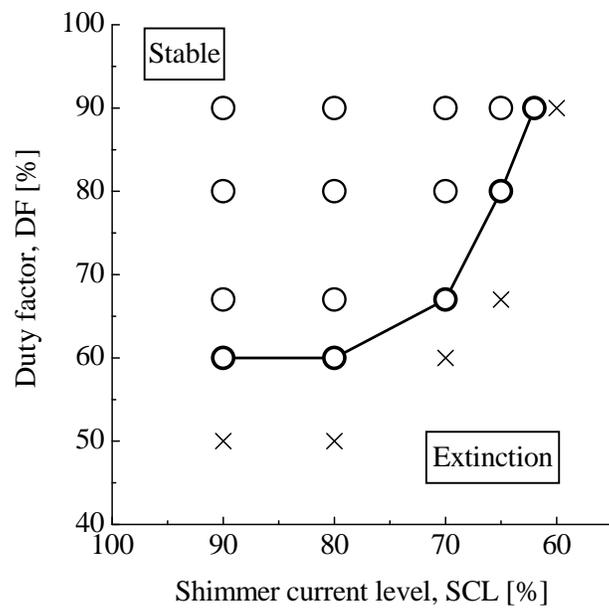
Figure 3: Stable operation region of Ar-O<sub>2</sub> PMITP at 20 kW.
