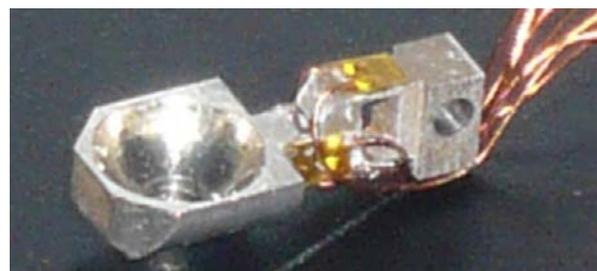
Fig.5. Manufactured clip and fit strain gages
