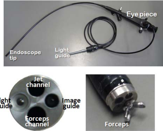
Fig. 2 Photographs of the newly designed endoscope
