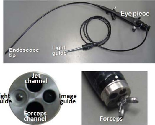
Fig. 2 Photographs of the newly designed endoscope
