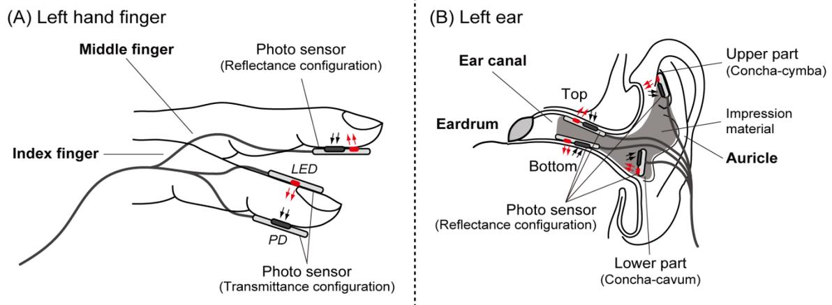
**Figure 1.** The placement of sensors for the measurement of NPV. Left hand finger; an index finger using the transmission type sensor as a reference; a middle finger using the reflection type sensor (panel A). Left ear; the top and bottom of the ear-canal, and the upper and lower part of the ear-auricle using the reflection type sensors (panel B).
