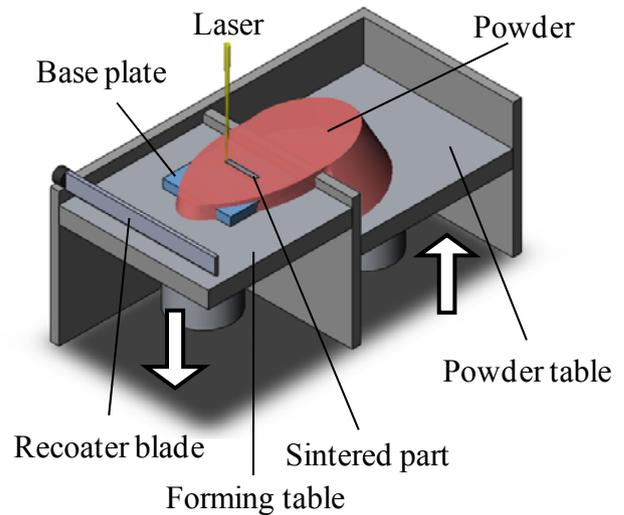
Fig. 1 Schematic illustration of laser sintering process
