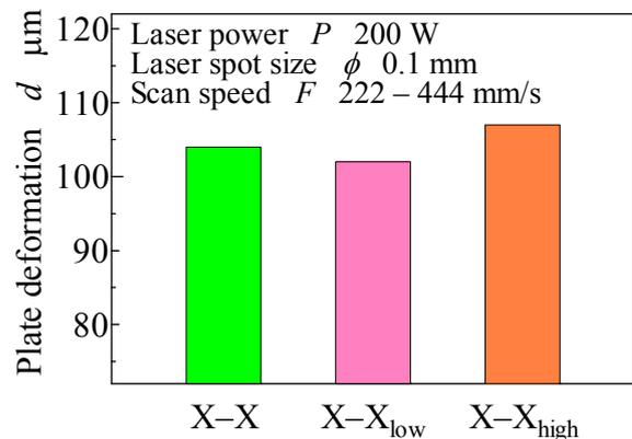
Fig. 10 Model deformation by different laser energy density
