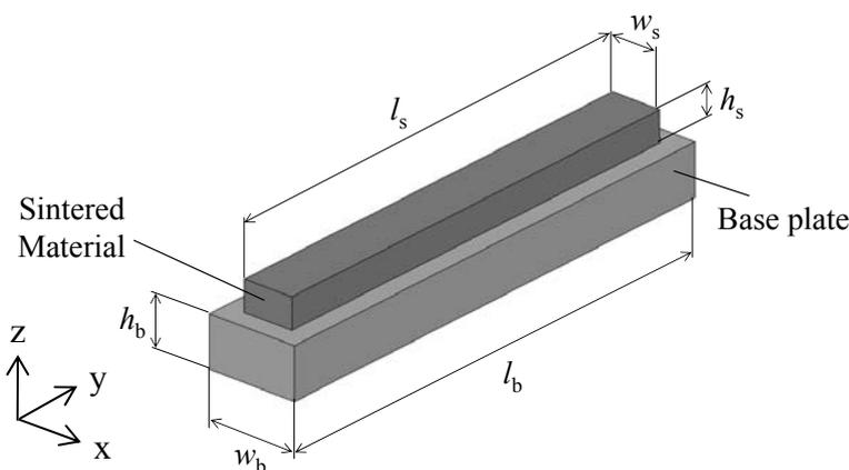
Fig. 2 Schematic illustration of sintered test model
