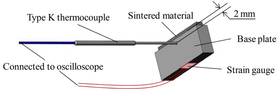
Fig. 4 Schematic illustration of temperature and strain measurement
