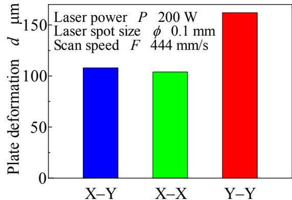
Fig. 8 Model deformation by different laser scan direction
