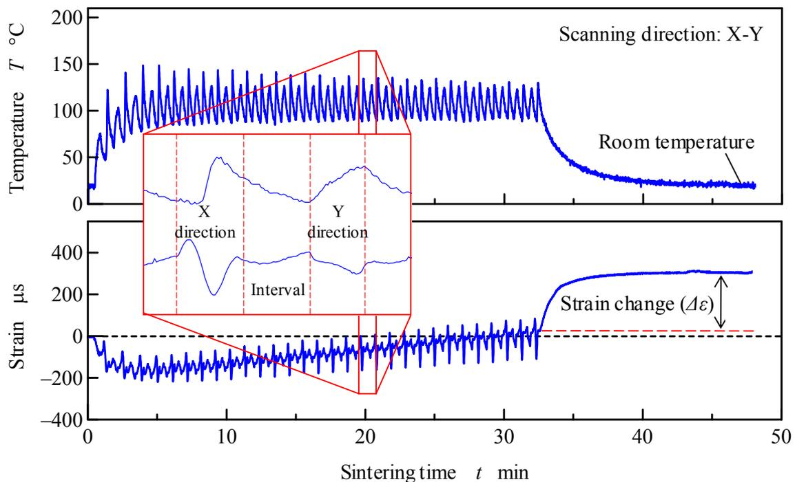
Fig. 6 Temperature and strain history during sintering process
