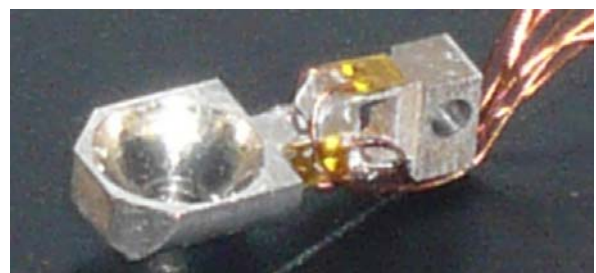
Fig.5. Manufactured clip and fit strain gages
