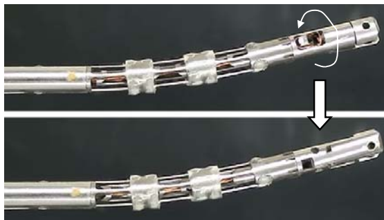
Fig.14. Rotation of the gripper at the end of flexed manipulator
